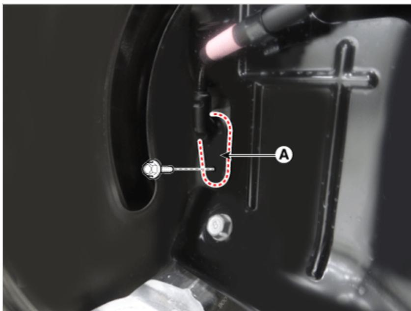
5. Remove the wheel speed sensor bracket (A).
