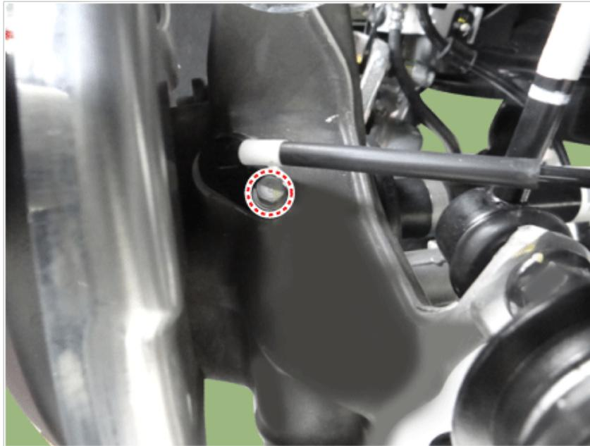
5. Disconnect the ECS sensor connector (A) and then remove the bracket (B).
