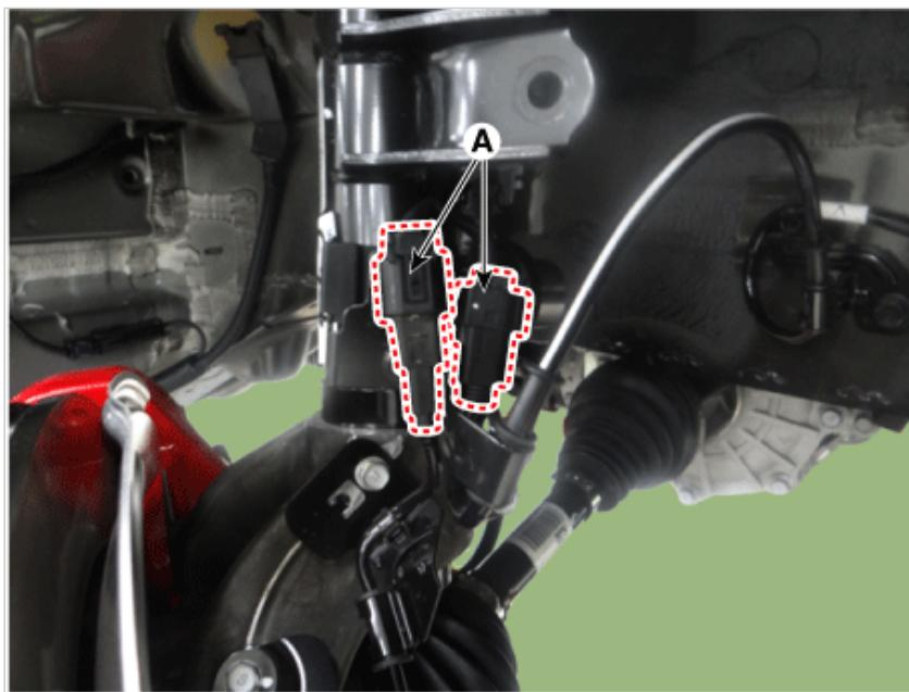
7. Remove the bracket (A) and then disconnect the connector (B).
